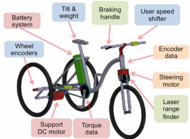
Figure 3 Tricycle subsystems
